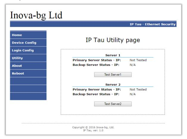
In **Utility** menu, connections to the servers can be tested. When the test button is clicked the device will send test messages to the server. If a backup server is enabled – the device will test this connection also.
