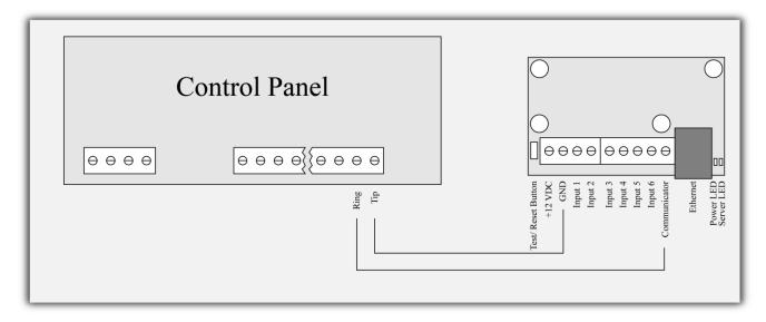
IP Tau has a built-in communicator/dialer receiver. It can receive data from each security panel with communicator/dialer option. Settings for the security panel (in some models additional settings may also need to be made):
