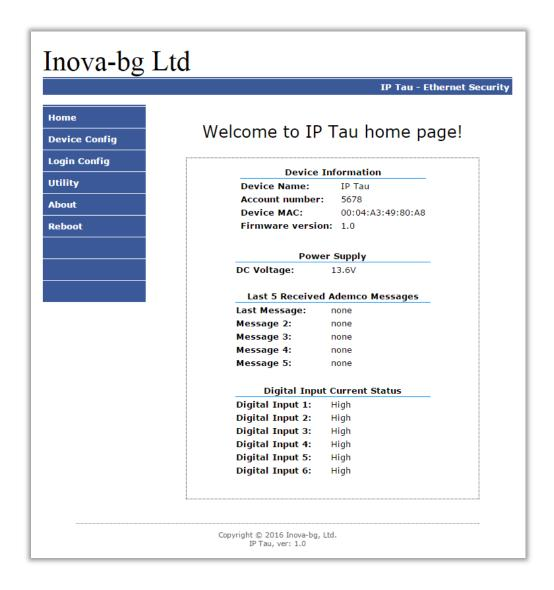
On the homepage you can find main information about the device, current status of the input voltage, last 5 messages received from the communicator and the current state of each digital input. Through the menu you could select one of the following actions:
