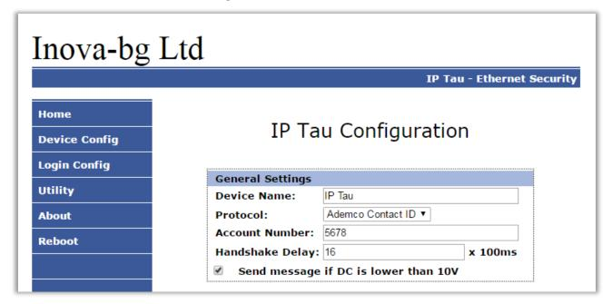
**Device Name** – Enter the name of the device. This value is used only for user convenience – to identify devices if you have more than one connected to one network. Maximum length -30 symbols.
