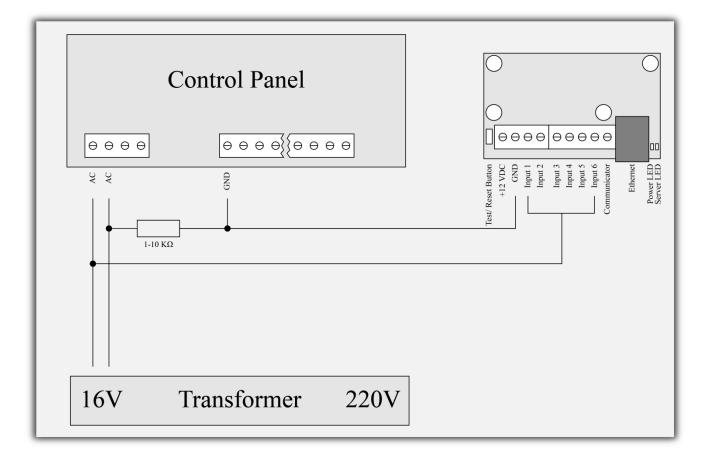
Each of the digital inputs could be used as a "Hardware AC" input. In this mode it will monitor the AC and generate a message for "AC Loss/AC Restore".
